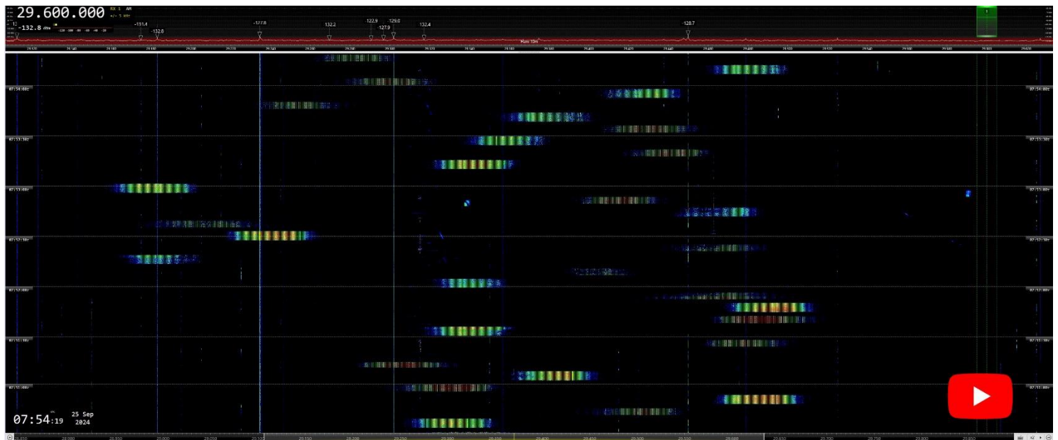
10 meters: OTHR IRN. BW ca 45 kHz. Alternating 333 sps and 695 sps bursts. Jumping after every burst
