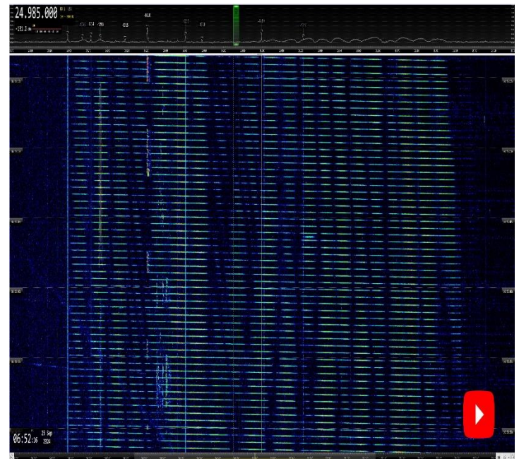
25000 kHz CF: CODAR-like radar. BW = 200 kHz. 2 pps
