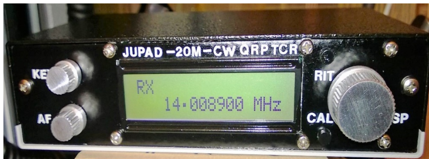
Home-made QRP (4W OUT PWR) 20m CW TRCVR
